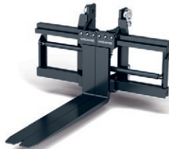
Carriage with kissing forks for steel handling
